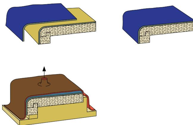
2. The laminate is bonded to the substrate in the area that will remain flat and is then postformed along the profile of the backing, while at the same time making it adhere to the rounded edge using a certain amount of pressure (a continuous process is recommended for mass production).
