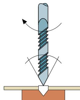
Drilling with milling cutter
